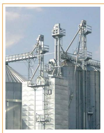
**PETKUS Bucket Elevators** are used for the vertical transport of bulk material in the industry and agriculture, like cereals, oil seeds, pulses, as well as for the transport of products in powder form.
