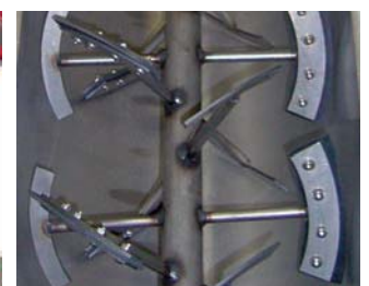
Secondary mixing unit
