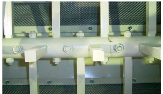
De-awner trough with a cover of moulded indent and the shaft with rectangular beater bears.
