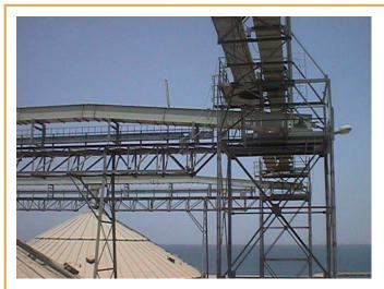
The PETKUS Troughed chain conveyors are very rigid constructions and well suitable for the conveyance of bulk material in the agriculture and industry, like cereals, oil seeds, pulses, as well as for the transport of products in powder form. The maximal achievable conveying length by using the standard equipment is 50 m. The increase of the conveying length is possible and needs to be calculated. The direction of the transport can be one-side, double side and reversible.
