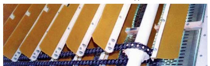
Sieve cleaning system - endless chain with plastic blades and rubber balls
